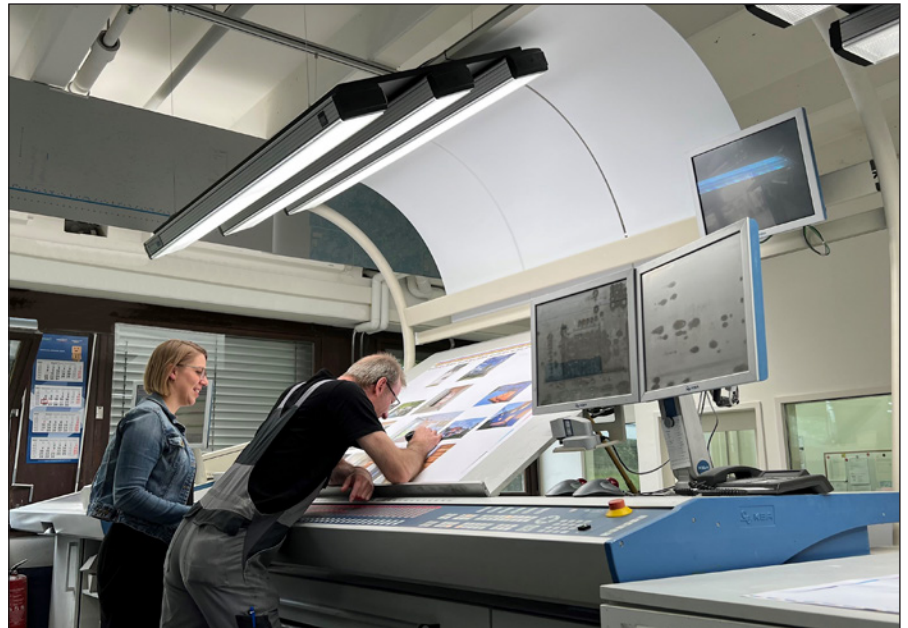
The Karl Grammlich offset printing company retrofit the luminaires in its existing press control console to the patented LED-based solution from JUST Normlicht.
